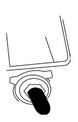
**Tow Switch:** The Tow switch is located in the front of the battery container. The switch can be seen clearly when the seat bottom is being opened by means of pulling the armrest forward. Pulling the switch to TOW (or OFF) will cut the power off and make the car stop.
