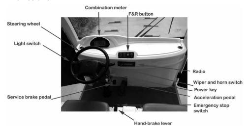
*Power key:* Controls the power supply of the whole vehicle. When the key is inserted into it and turned clockwise, it will switch on the lights, horn, and the control system; when the key is turned back, the power will be switched off.
