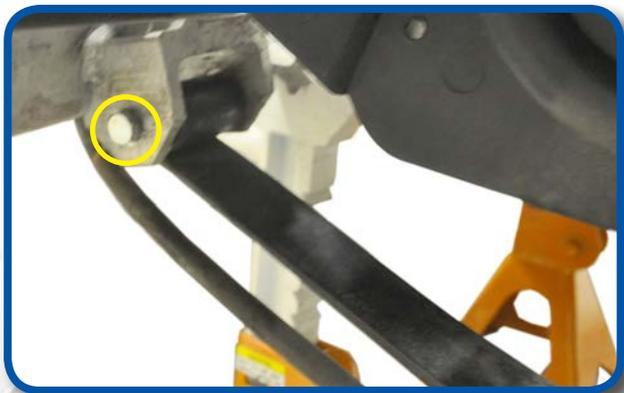
Use the jack to lower the rear end. Reposition spring above the axle and remount to factory mounting points using retained hardware from Steps 21 and 22.
