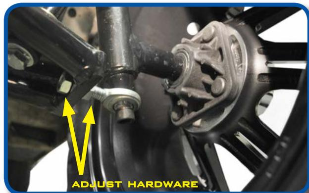
To adjust camber (the vertical tilt of the wheels) to 90 degrees using the two nuts on the bottom heim joint (B).
