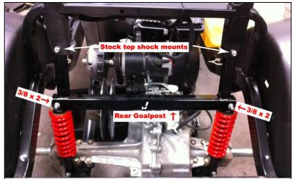
The rear goalpost mounts to the stock TOP shock mount as shown, this part does NOT mount to the bottom stock shock mount
