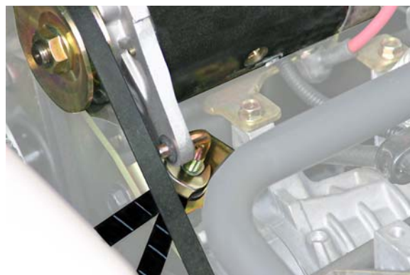
Fig. 36 Adjusting the Belt Tension
