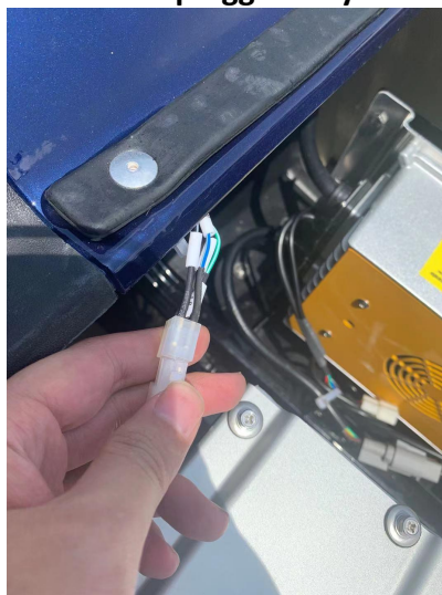
4 Pin square connector plugged to vehicle programming interface on the wiring harness
