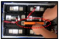
5. Re-connect the battery module's connectors.
