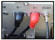
8. Press the "SW" switch to activate the BMS, then test the cart.
