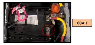
4.2.3 Take out the whole BMS mounting board with BMS & golden pre-charge resistor.
