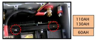
For 60AH lithium pack, also need to loosen this cable (from solenoid to module's negative pole) .
