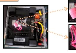
Note: Must unplug [P+] connector first, then unplug [P-] connector (For 60Ah)
