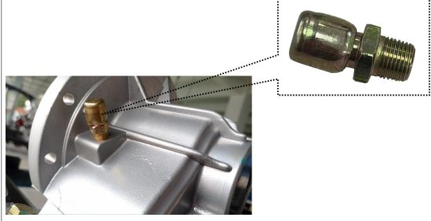
2.Reduce the amount of differential gear oil, the required amount is 650 ml (22 oz). The size of oil is GL-4 85W-90.
