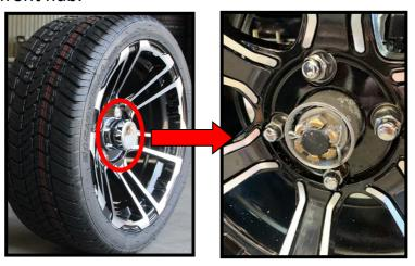
1.1.2 Inspect the inner side of center dust cap and the cotter pin fixing the slotted nut to check whether there is any scratching marks or chips.
