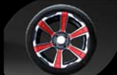
14" Alum Wheel with black insert/215/35R14 Radial DOT Tire
