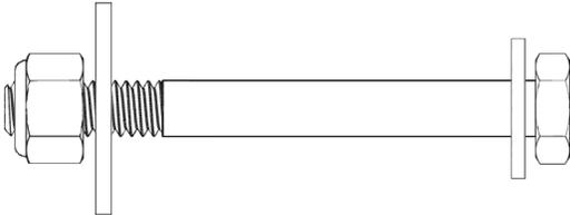
1/4" X 2-1/2" Hex Bolt - 1/4" Flat Washer - 1/4" Fender Washer - 1/4" Nylock Nut
