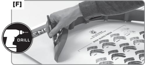
**F]** Hold the Fender Flare secure and mark hole locations. Drill 5/16" holes at all marks.
