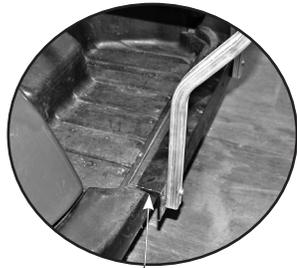
**1)** Rest the Bumper Angle/Cargo Bed Upright Support Assembly on top of the bumper.
