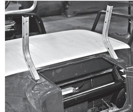
Use the original hardware from the bag rack assembly (removed in step 1).
