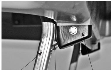
Rear Strut    Drain Tube    Rain Cup
