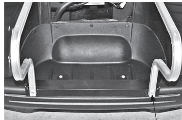
Attach the cargo bed frames to the the Bumper Angle. Attach to the second hole from each outside edge of the Bumper Angle. Hand-tighten hardware only.
