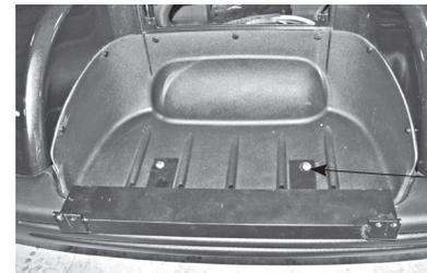
**2)** Place the bumper angle over the bumper and mount it to the car using the holes exposed from step 1.
