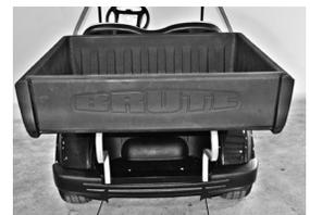
**2) Fully tighten hardware connecting the cargo bed frames to the bumper angle.**
