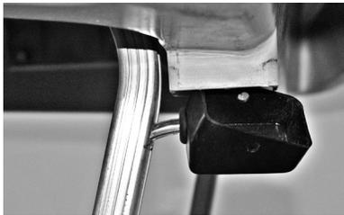
**1) Choose the correct drain cup ("D" is driver & "P" is passenger) and insert the drain tube into the hole on back of the corresponding rear strut. Work the drain tube down into the rear strut, until the rain cup is in position to be easily mounted over the down spout in the top. (NOTE: make sure that the drain tube is flush with the inside of the rain cup and does not pull out of the rain cup during installation).**
