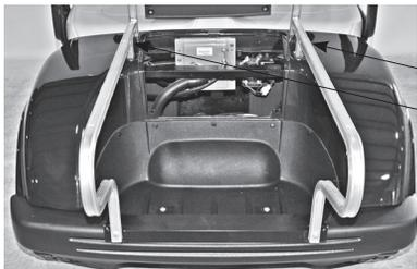
**1)** Place cargo bed frames into holes where the bag rack was removed.
