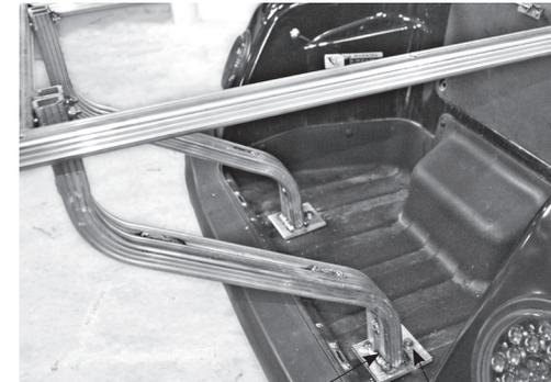
Mount each cargo bed support to the car, using the holes that were drilled in the bagwell floor from STEP 1C.
