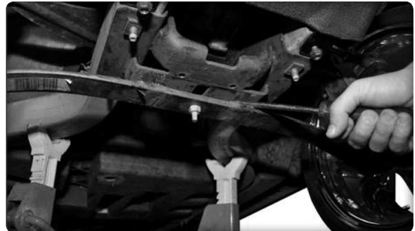
Pry the leaf spring away from the cart to allow enough clearance for the lift bar.
