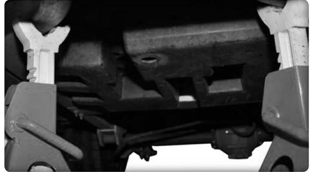
Place RUN/TOW switch in TOW position. Chock wheels and lift cart. Place cart on jack stands as shown.
