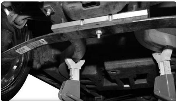
Place lift block between leaf spring and frame.
