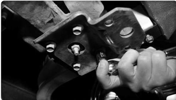
Remove the plate by removing the four factory bolts as shown.
