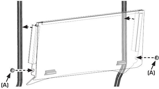
Insert grommets into slots on Windshield, then snap Extrusions & Windshield onto front frame.
