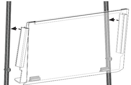
Snap Extrusions & Windshield onto front frame, then slide until Windshield sits on grommet. ↓
