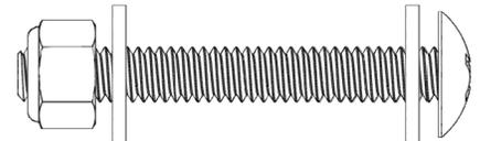
1/4" X 2" Truss Bolt - 1/4" Flat Washer (x2) - 1/4" Nyloc Nut
