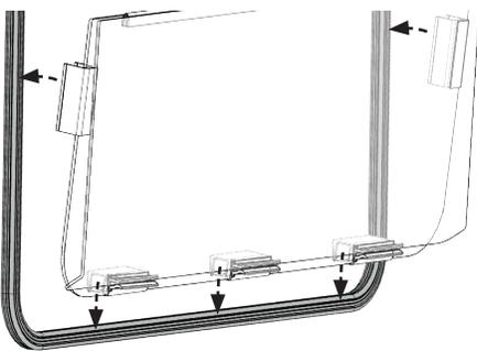
Push in and down at the same time to snap the Extrusions & Windshield onto the front frame.
