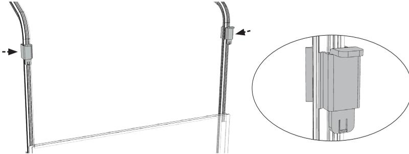
Snap Upper Latches onto front frame.
