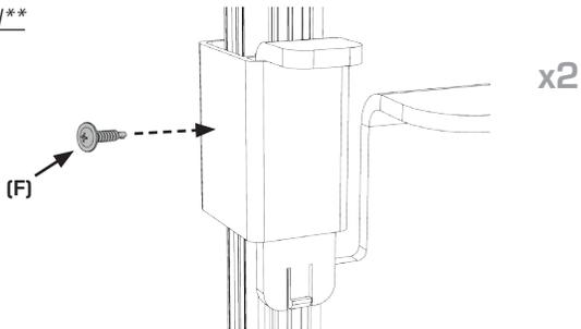
Optional: Use self-tapping screw and drill to permanently install Upper Latches.
