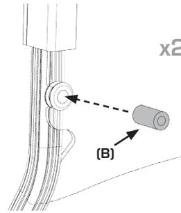
Slide Extrusion & Windshield until grommet aligns with hole in frame, then insert spacer. ↑ ↓
