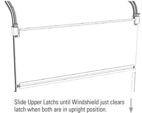
Slide Upper Latches until Windshield just clears latch when both are in upright position.
