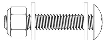
1/4" X 1-1/2" Truss Bolt - 1/4" Flat Washer (x2) - 1/4" Nyloc Nut
