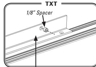
Top Frame mounts to inside of TXT Bracket
