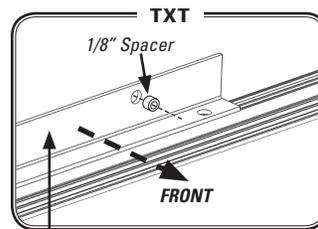
Top Frame mounts to Front Side of TXT Bracket
