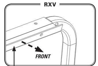
Top Frame mounts to Front Side of RXV Bracket
