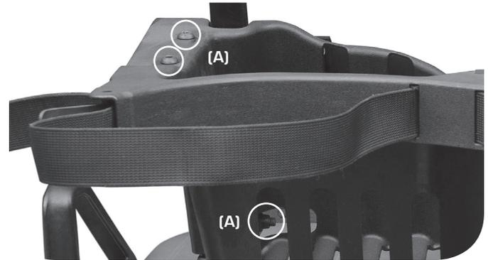
Attach the Universal Seat Back Plates to the Seat Back Supports using 1/4" x 1-3/4" FHP Bolt, 1/4" Flat Washer (back), and 1/4" Nyloc Nut (2x both sides – through top and bottom holes marked RXV).
