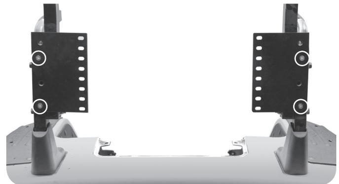
Install Seat Back Cushion (A) to Seat Plates (see Section 3 for example). Then, complete your installation by reinstalling the Bag Holder/Sweater Basket Assembly using the factory hardware (B).
