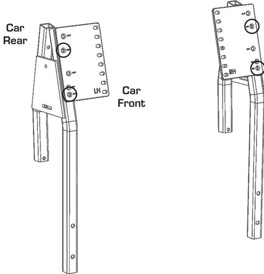
Attach the Rear Seat Back Plates to the Seat Back Supports using a 1/4" x 1-3/4" FHP Bolt, a 1/4" Flat Washer (back), and a 1/4" Nyloc Nut (2x both sides – through the upper set of holes marked RXV).
