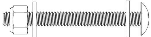
1/4" X 2-1/2" Truss Screw - 1/4" Flat Washer - 1/4" Nylock Nut
