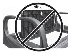
**DO NOT PUSH OR FORCE THE LID PAST 90° BEFORE SEAT BASE & SEAT BACK CUSHION ARE INSTALLED ON THE CAR**
