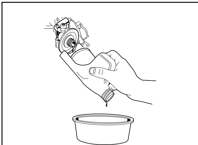
Figure 39 Remove Engine Oil Filter
