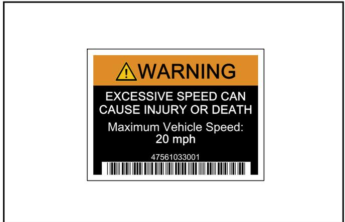
6. Decal, Excessive Speed Warning (Gasoline Vehicles Only. Located Under Floor Board.)
