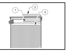
Figure 25 Gasoline Battery Electrolyte Level
