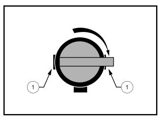
Figure 15 Fuel Shut-off Valve – Closed Position
