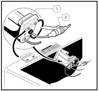
Figure 23 Receptacle Fuse Link
