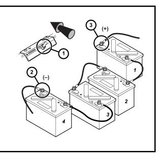
Figure 2 IQ System Electric Vehicle - 12-Volt Battery Configuration
