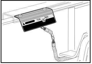
Figure 10 Tow/Run Switch - IQ System
