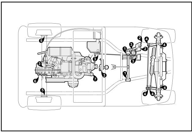
Figure 19 Lubrication Points – Gasoline Vehicles
