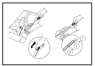
Figure 26 Engine Oil Level Check
