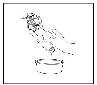
Figure 28 Remove Engine Oil Filter
