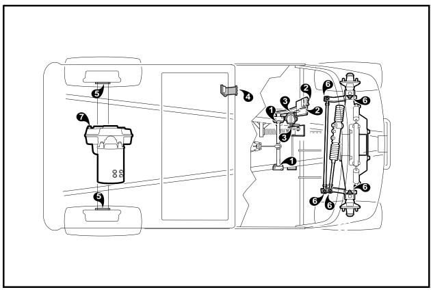
Figure 18 Lubrication Points – Electric Vehicles
