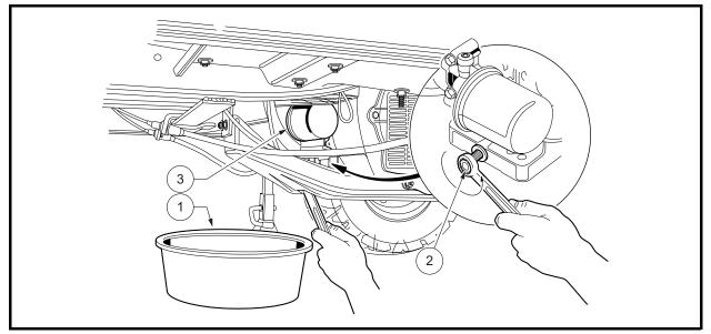
Figure 27 Engine Oil Drain Plug and Pan
