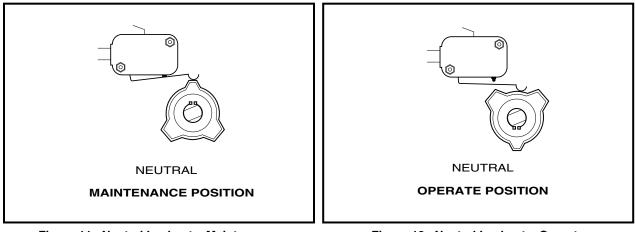
Figure 11 Neutral Lockout – Maintenance
