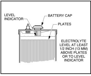
Figure 20 Electric Battery Electrolyte Level
