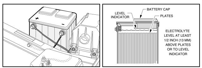
Figure 24 Battery – Gasoline Vehicle
