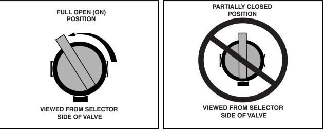
Figure 16 Fuel Shut-off Valve – Open Position
