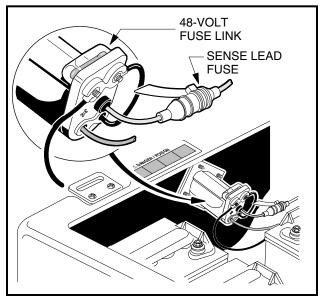
Figure 23 Receptacle Fuse Link
