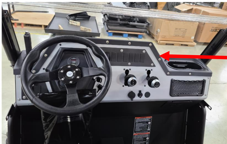
Figure 4: Removing Black Instrument Panel Cover
