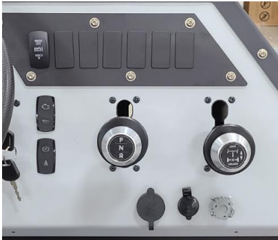
Figure 15: Remote Winch Capped Off
