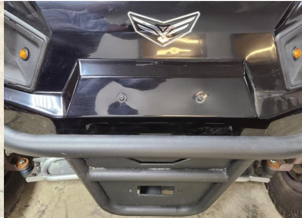
Figure 3: Removing Two Hood Fasteners
