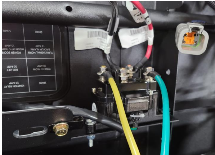
Figure 8: Winch Contactor Mounting Location
