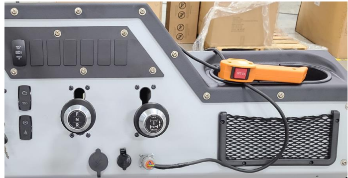
Figure 16: Remote Winch Switch hooked up
