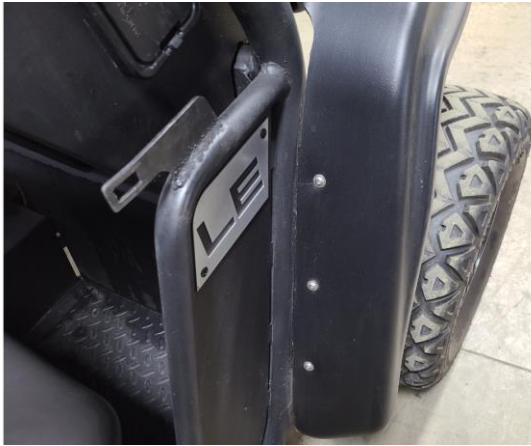
Figure 2: Removing Three Fender Fasteners
