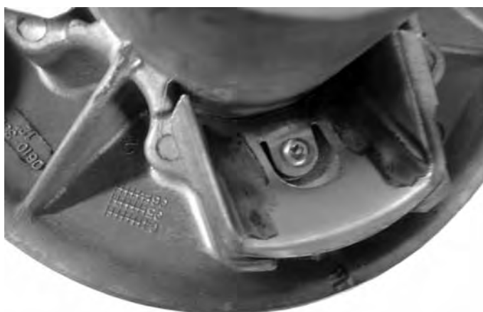
the sliding flange ramps once cleaned
