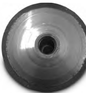
sliding flange before cleaning
