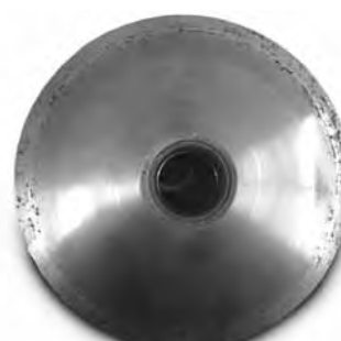
sliding flange after cleaning
