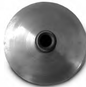
fixed flange after cleaning
