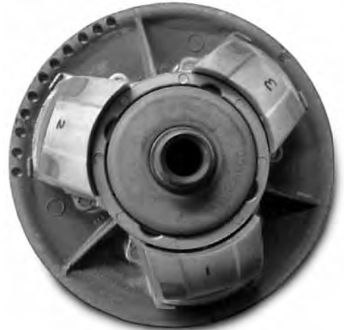
Pulley with the cap are removed
